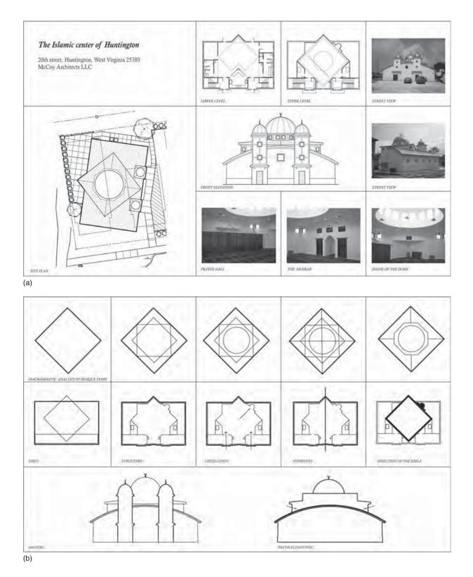
Figure 4.13 The Islamic Center of Huntington: (a) formative concept; (b) analytic diagrams. (Graphics by Raheel Ahmad; designed by McCoy Architects LLC)
